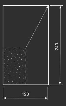
With individual elements of up to 240 cm x 120 cm and up to 75 light points per square metre, a versatile facade design is possible.
